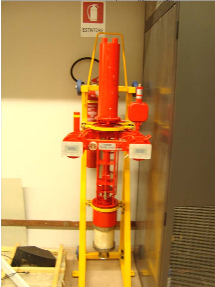
45 MW pulsed S-band klystron (Thales TH2132A)
