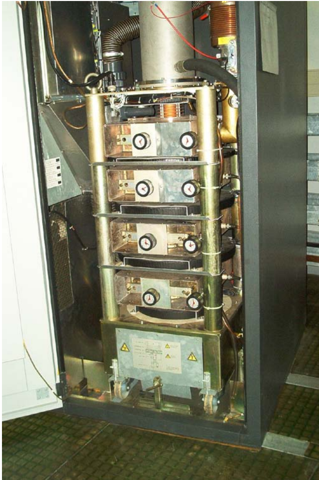
External cavities UHF Klystron used at Elettra 60 kW cw 500 MHz (E2v 2672BCD))
