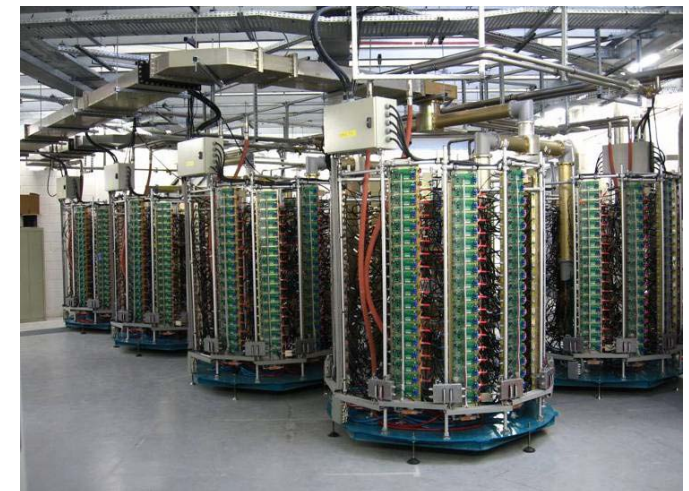
Solid state amplifier towers at SOLEIL (352 MHz)
