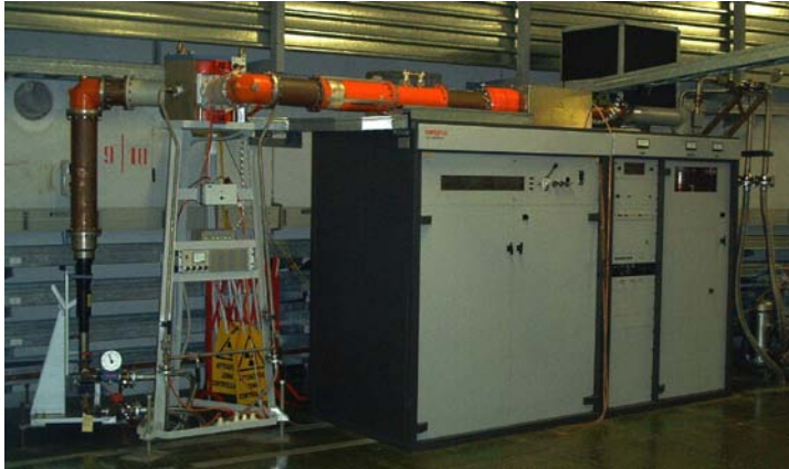
60 kW cw 500MHz klystron based amplifier at Elettra
