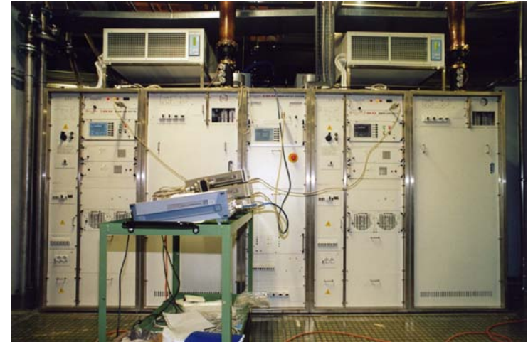
150 kW cw 500MHz combined IOTs based amplifier at Elettra
