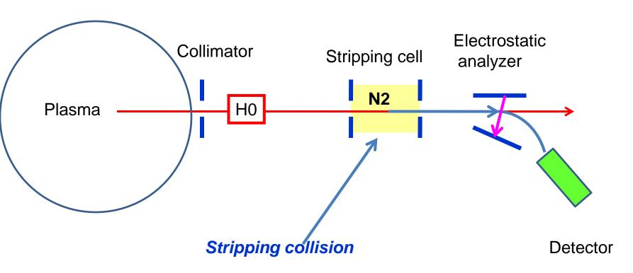
fast H<sup>0</sup> + slow N2 => fast p + ...... Resulting fast proton has almost the same energy and momentum as primary fast neutral
