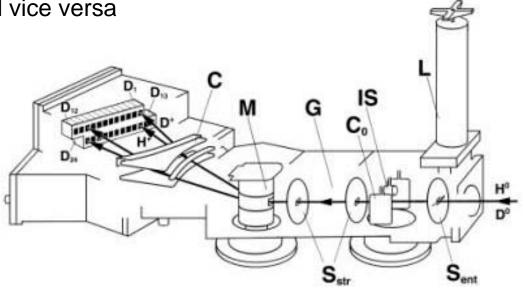
12 channels for hydrogen atoms, 12 channels for Deuterium atoms Energy spectrum of hydrogen and deuterium atom is measured simultaneously!
