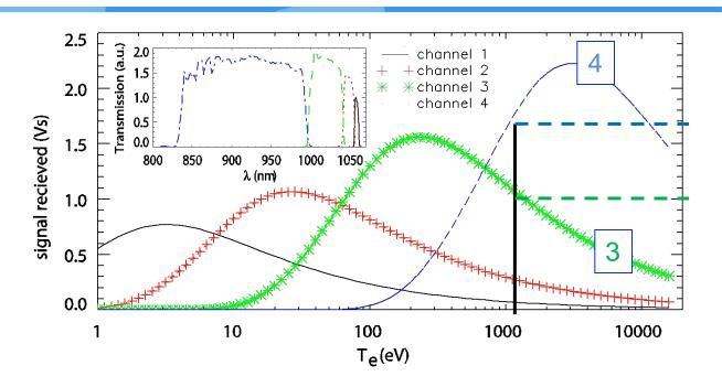
Electron temperature is derived from the ratio of signals from individual channels
