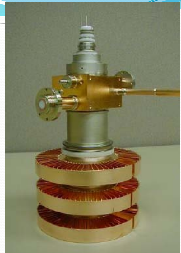
Ka band Multi Stage Depressed Collector (MSDC) EIK with a efficiency in excess of 50%
