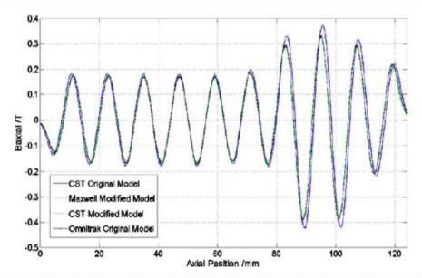
1D distance vs axial magnetic field graph along the beam tunnel axis obtained from CST-PS, Maxwell<sub>3</sub>D and Omnitrak
