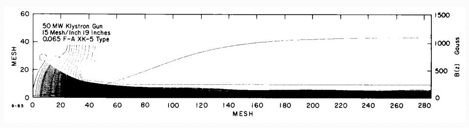
Calculated electron trajectories with magnetic field.
