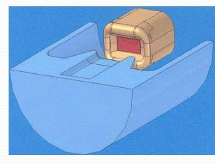
Sheet beam gun with 2:1 cathode aspect ratio
