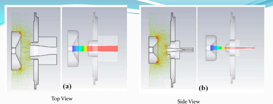
Electrostatic field vector plot and spatial particle distribution of the sheet beam gun in CST-PS. The beam voltage is 54kV and beam current is 2A.
