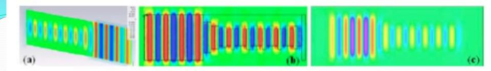
Axial magnetic field distribution from (a) CST-PS, (b) Maxwell and (c) Omnitrak
