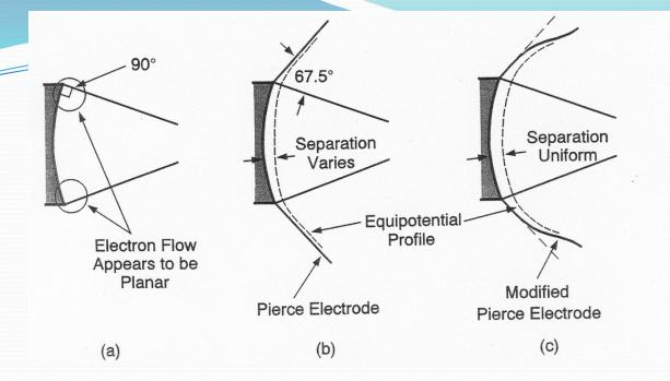
Modification of Pierce electrodes to produce spherical equipotential profiles
