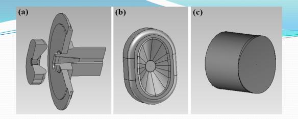
Cathode, Anode and Focus electrode of a WSBK in UCDavis
