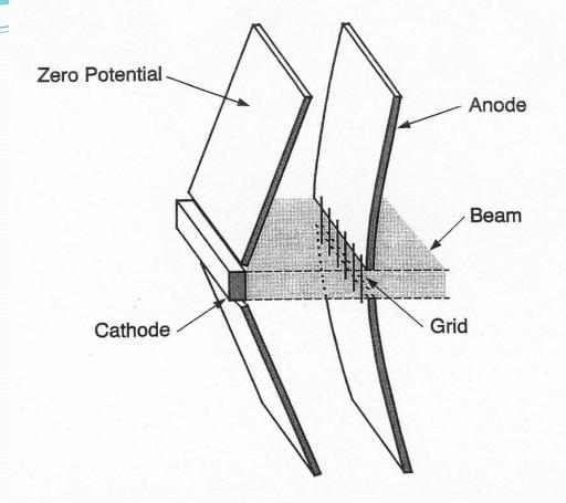
Electron gun for producing rectilinear electron flow
