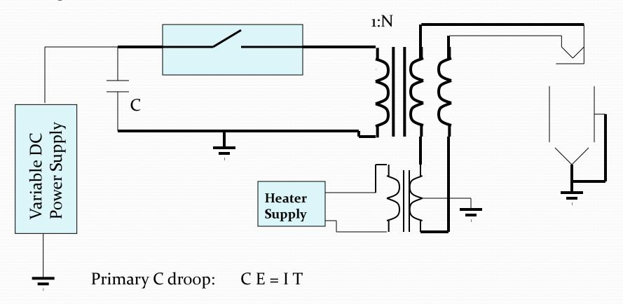
Rise time of pulse is mainly a function of Pulse Transformer
