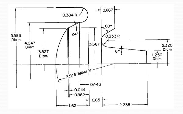
The electron gun is a critical portion of the design due to the high operating voltage (315 kV). Figure schematically illustrates the Pierce electron gun design. The high peak voltage gradient (174 kV/cm) and long voltage pulse duration (6  $\mu$ s) increase the possibility of voltage breakdown. However, it is reported that following careful selection of electrode materials, extensive polishing and proper conditioning that fewer than two high voltage breakdowns in an eight hour shift occur.
