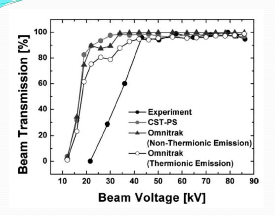
Beam voltage vs transmission graps obtained from experiment and simulation (CST-PS and Omnitrak)
