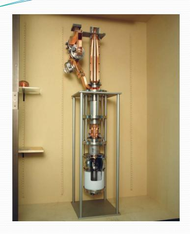
It shows a photograph of a partially cutaway klystron tube in SLAC. It can produce 65 MW output at a beam voltage of 350 kV and a beam current of 414A. An efficiency of 46% is achieved with a gain of 53 dB.
