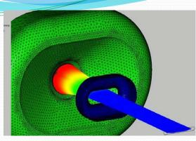
The NLC 75-MW sheetbeam klystron design
