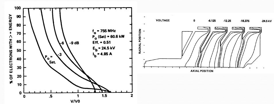
Calculated energy distribution of the spent beam for the VKP-7555 Klystron.
