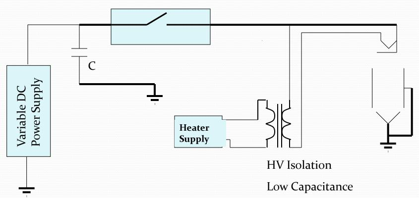
Pulse droop: C E = I T C is filter cap, T is pulse width, I is beam current
