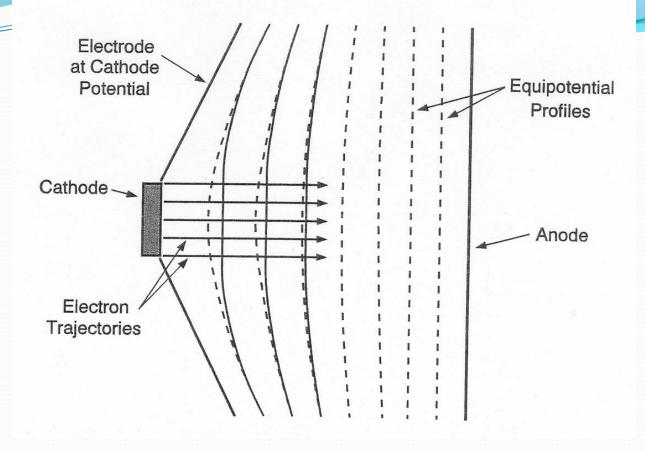
Straightening of equipotential profiles in electron beam
