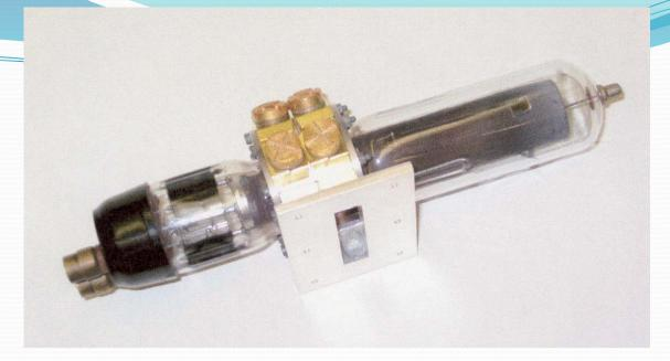
The EMI CV-150 (original UHF resonant cavity)
