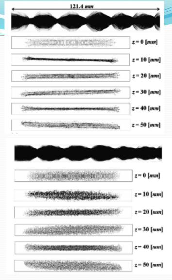
Electron beam distribution in wide and thin direction at several positions with o and 0.16 eV transverse temperature
