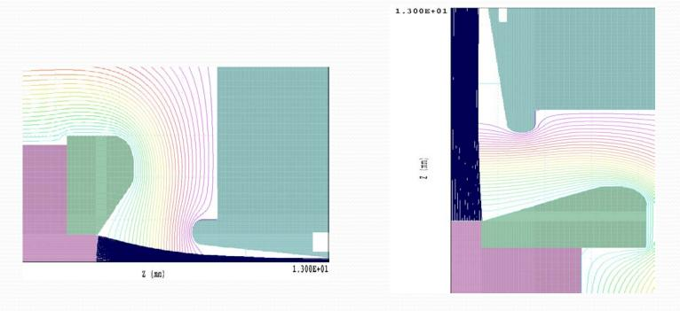
Omnitrak simulations of the beam focus
