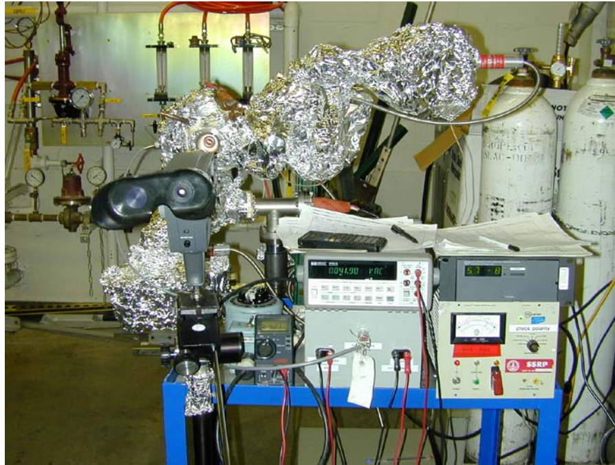
Pyrometric measurement after cleaning and baking
